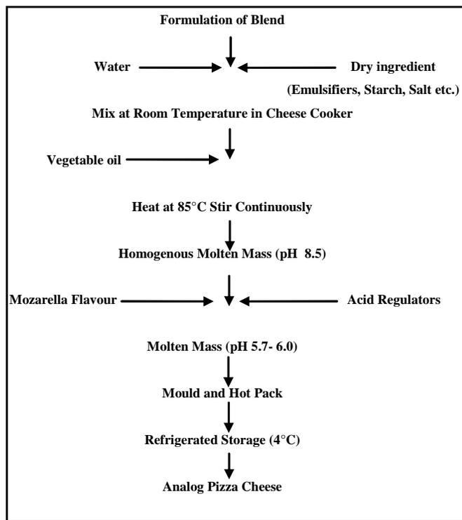
Fig. 2 : Flow diagram for manufacturing processes of cheese analogs
