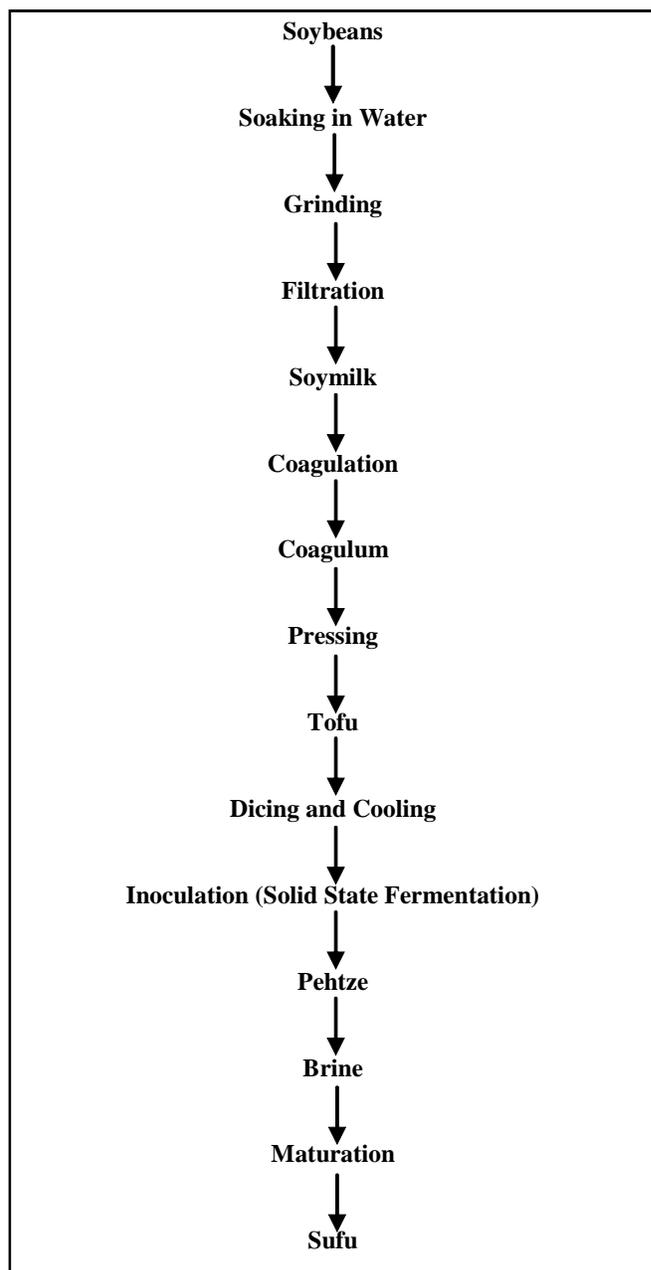
Fig. 3 : Schematic diagram for production of soft tofu
